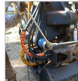
Torque multiplier used for machine nut tightening
