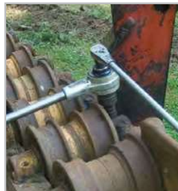
Torque multiplier used on tracks
