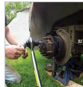
Torque multiplier used for lug nuts
